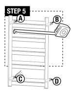
**STEP 5:** Use a tape measure to measure the distance between the center points of each wall bracket tube; record the distances between points AB, AC, CD, and BD. Mounting point C will determine electrical box location. See Electrical Assembly in following instructions.
