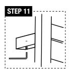
**STEP 11:** As shown in the picture, install the set screws (c) into the hole of all the tubes (a and b) using the allen wrench; fix the tube (a) onto the mounting bracket (g).
