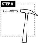
**STEP 8:** Use a hammer to knock plastic drywall anchor (f) into wall completely.
