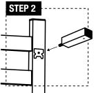
**STEP 2:** Use the short mounting screw (d) to fix the mounting tube (a) to the threaded metal pad on the vertical bar on the back of the towel warmer.
