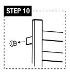
**STEP 10:** Install the tube (a) onto the bracket (g).
