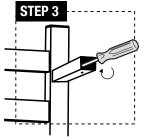
**STEP 3:** Screw down the short mounting screw (d) with a screwdriver. Note that the set screw of the tube (a) should point towards the floor when the towel warmer is wall mounted. Fix the remaining two mounting tubes (a) to the vertical bars with threaded metal pads by repeating Step 1-3.
