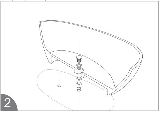
3. After placing the bathtub on its side and fixing it, then install the bathtub drain bounce device.
