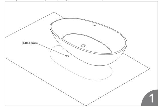
2. If the height is not enough, you can raise the height of the bathtub installation plane, or dig a sink with a depth of about 50mm on the ground to place the drainage device.
