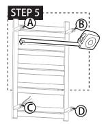
STEP 5 Use a tape measure to measure the distance between the center points of each wall bracket tube; record the distances between points AB, AC, CD, and BD. Mounting point C will determine electrical box location. See Electrical Assembly in following instructions.
