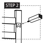
STEP 2 Use the short mounting screw (d) to fix the mounting tube (a) to the threaded metal pad on the vertical bar on the back of the towel warmer.
