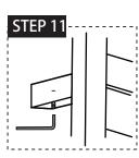
STEP 11: As shown in the picture, install the set screws (c) into the hole of all the tubes (a and b) using the allen wrench; fix the tube (a) onto the mounting bracket (g).
