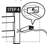
STEP 4 Guide the electrical cord through the electrical connection mounting tube (b) and use the long mounting screw (e) to tighten the electrical connection mounting tube to the vertical bar.
