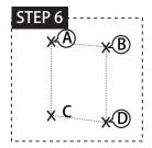
STEP & Mark A, B, C, and D according to the data from Step 5; It is suggested that this product be installed at least 23.5 inches (59.69 cm) above floor level. (WARNING: The electrical connection should avoid all water). This mounting location must comply with all local building and electrical codes.
