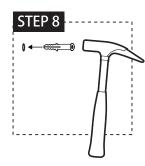
STEP & Use a hammer to knock plastic drywall anchor (f) into wall completely.
